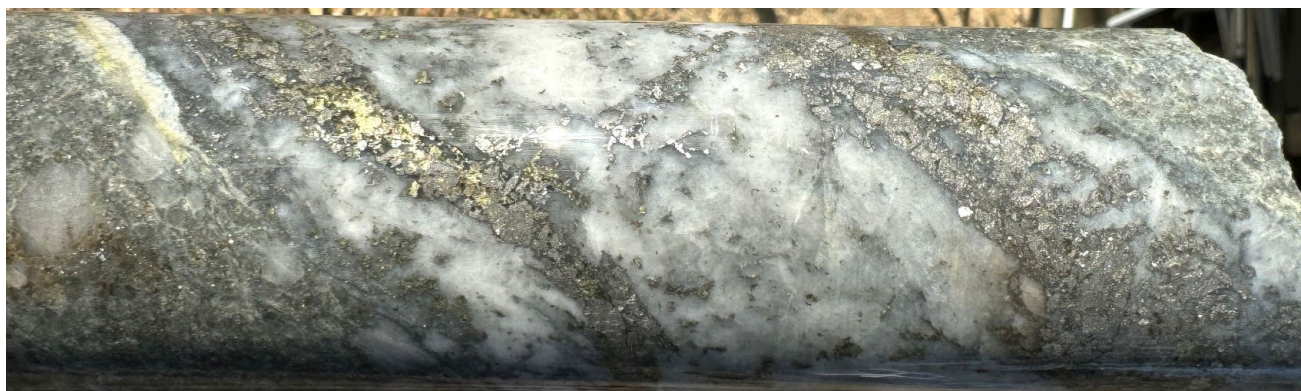
Figure 8: Photo of a quartz-pyrite-chalcopyrite-pyrrhotite-arsenopyrite vein intersected in drilling at Graceland (GRNDD00001, 209.1m, Assay results pending, expected in the December quarter). *Visual estimates of mineral abundance should never be considered a proxy or substitute for laboratory analyses where concentrations or grades are the factor of principal economic interest. Visual estimates also potentially provide no information regarding impurities or deleterious physical properties relevant to valuations.
