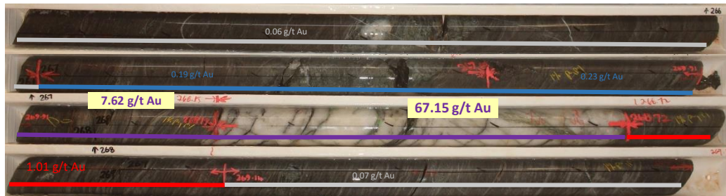
Diamond drill core photo 18WDDD0024 with gold assays – total intercept 8.14m at 7.11 g/t Au
