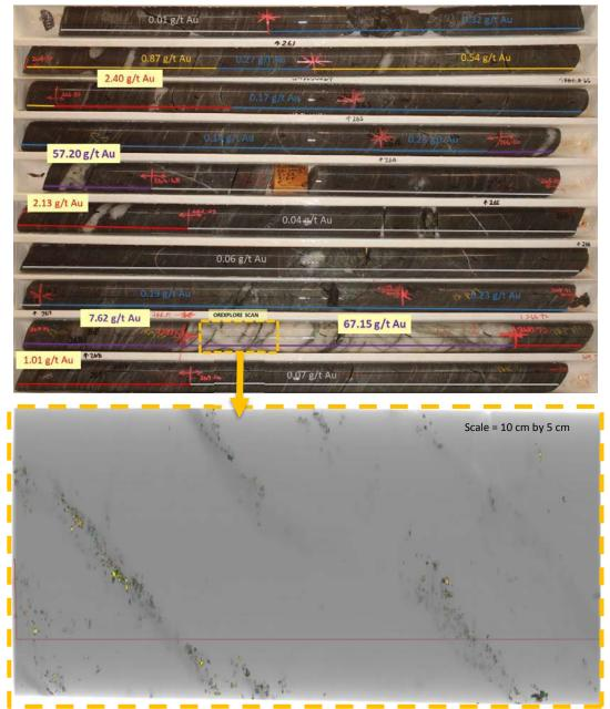
Figure 5: Diamond drill core photo (top) and Orexplore image (bottom) from hole 18WDDD0024. The downhole orientation mark is represented by the black line in the core photos and in the Orexplore image by the red line (268.22 to 268.32 metres). Gold is represented by bright yellow and pyrite by the green and darker colours, quartz is grey. The Orexplore image is rotated to look along the lamination planes within the quartz vein demonstrating the association with gold.
