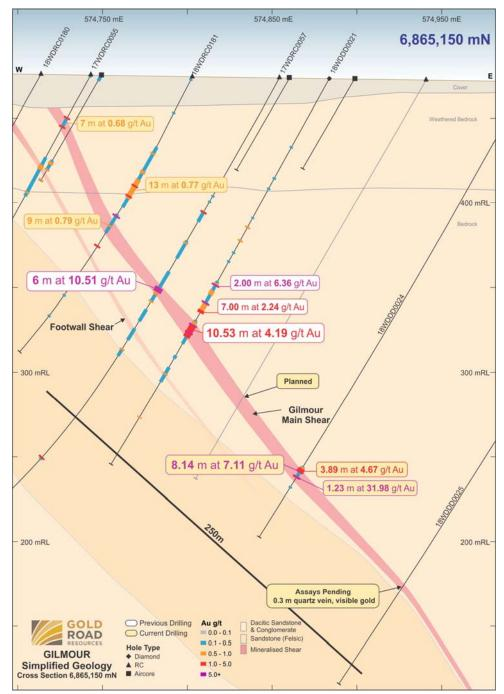
Figure 4: Cross section of the Gilmour Deposit showing interpreted geology and selected intersections
