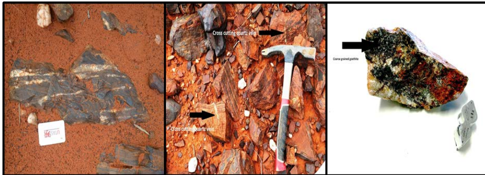
Subcrop/outcrop and surface float Banded Iron Formation (BIF) with quartz veining (Left and middle), and quartz vein sample (right) showing weathered sulphides after pyrite-galena observed during recent mapping
