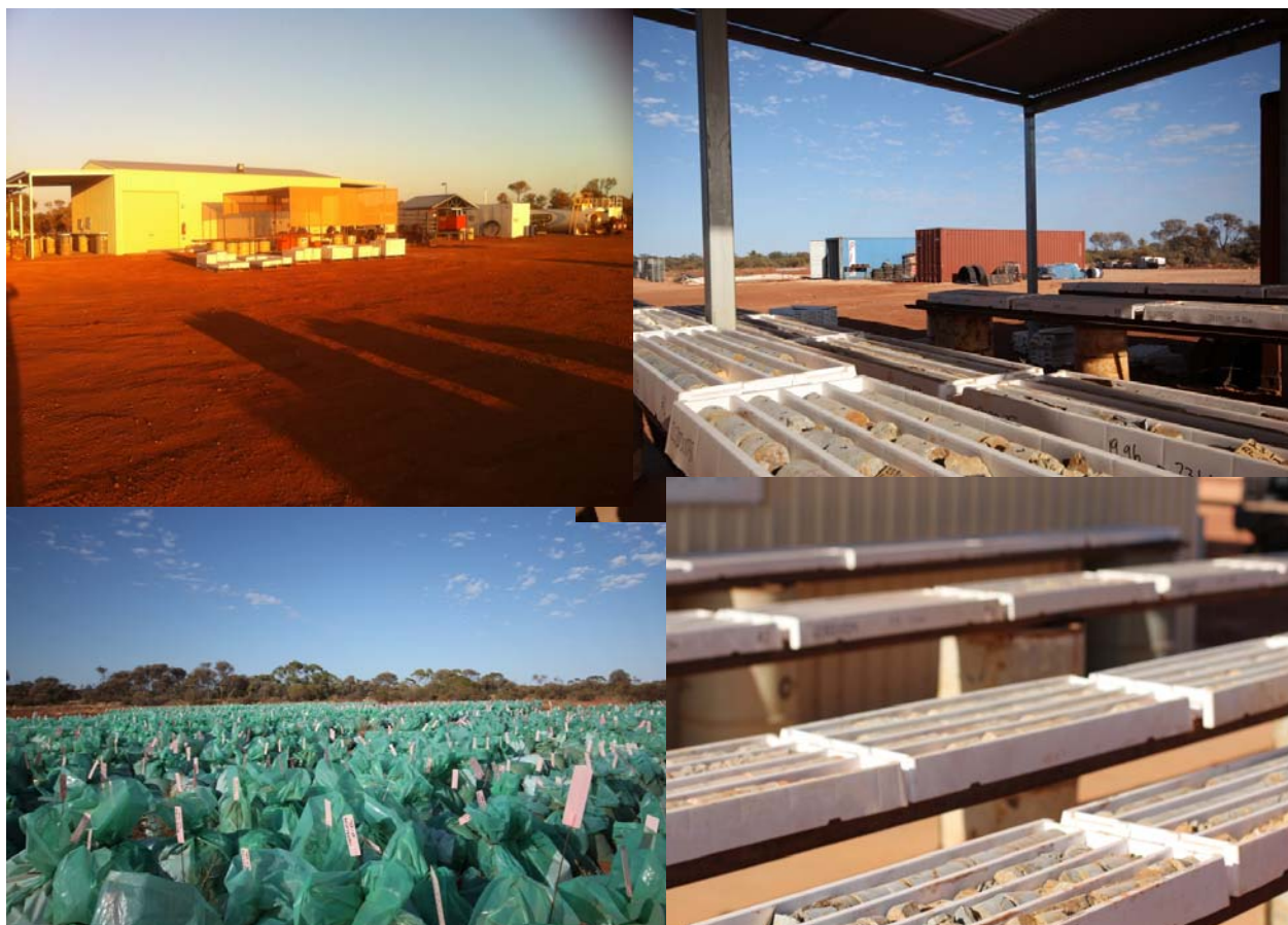
Photos Clockwise from Top Left - core cutting area; core awaiting cutting; cut core; sample bag field
