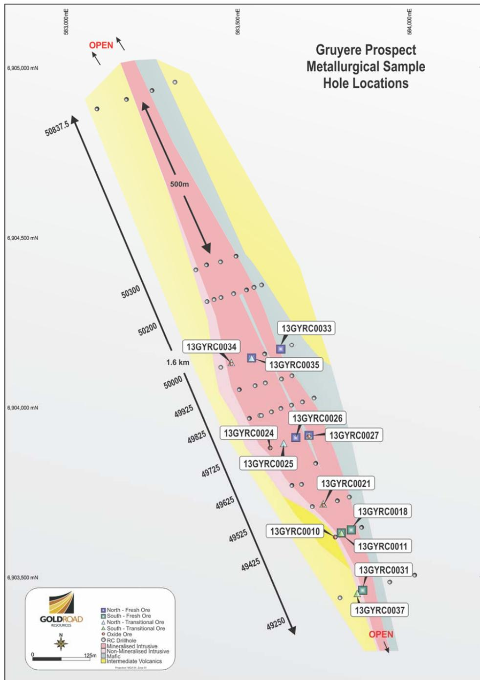
Figure 1: Gruyere plan projection illustrating location of RC holes sampled for Metallurgical testing composites (Appendix 1).
